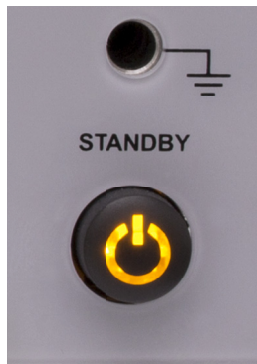
Figure 3-2. Indicator Glows Amber when Converter is In Standby
