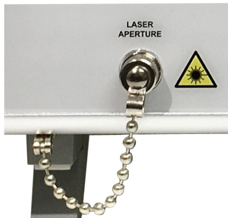
Figure 3-4. MN4775A-0040 Laser Aperture and Cap.
