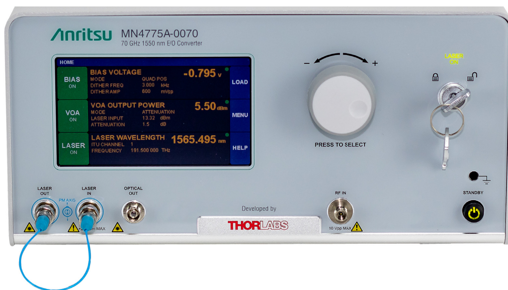
Figure 3-13. MN4775A-0070 E/O Converter Front Panel
