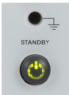
Figure 3-6. Indicator Glows Green when Converter is Fully Enabled
